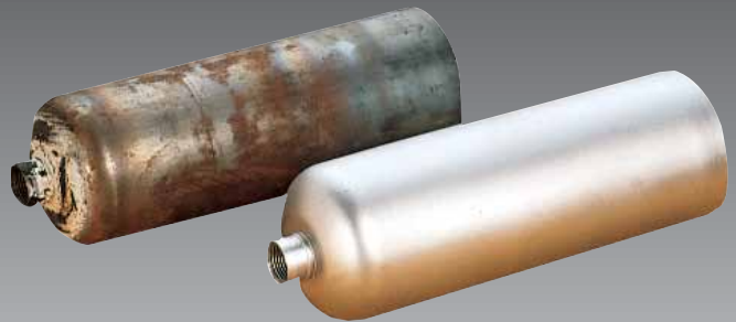
Cylinder surface profiled with aluminum oxide
